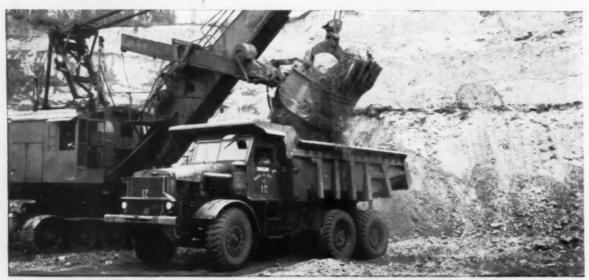
Rear-Dumps of 40 and 50-ton capacities are powered by two engines providing a total of 470 to 670 h.p.—each engine drives one of the tandem axies through a separate torque converter and semi-automatic transmission.
